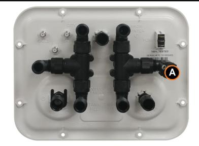
To connect plumbing line running to pump inlet, screw swivel fittings onto diverter valve ( (TO PUMP) as illustrated. This line will run directly to "IN" side of water pump.
